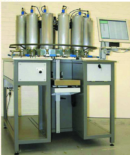
Hue Color Systems recently introduced the CD-14 Carousel Ink Dispensing System for the most accurate color matching of UV and conventional offset inks in cartridges.
